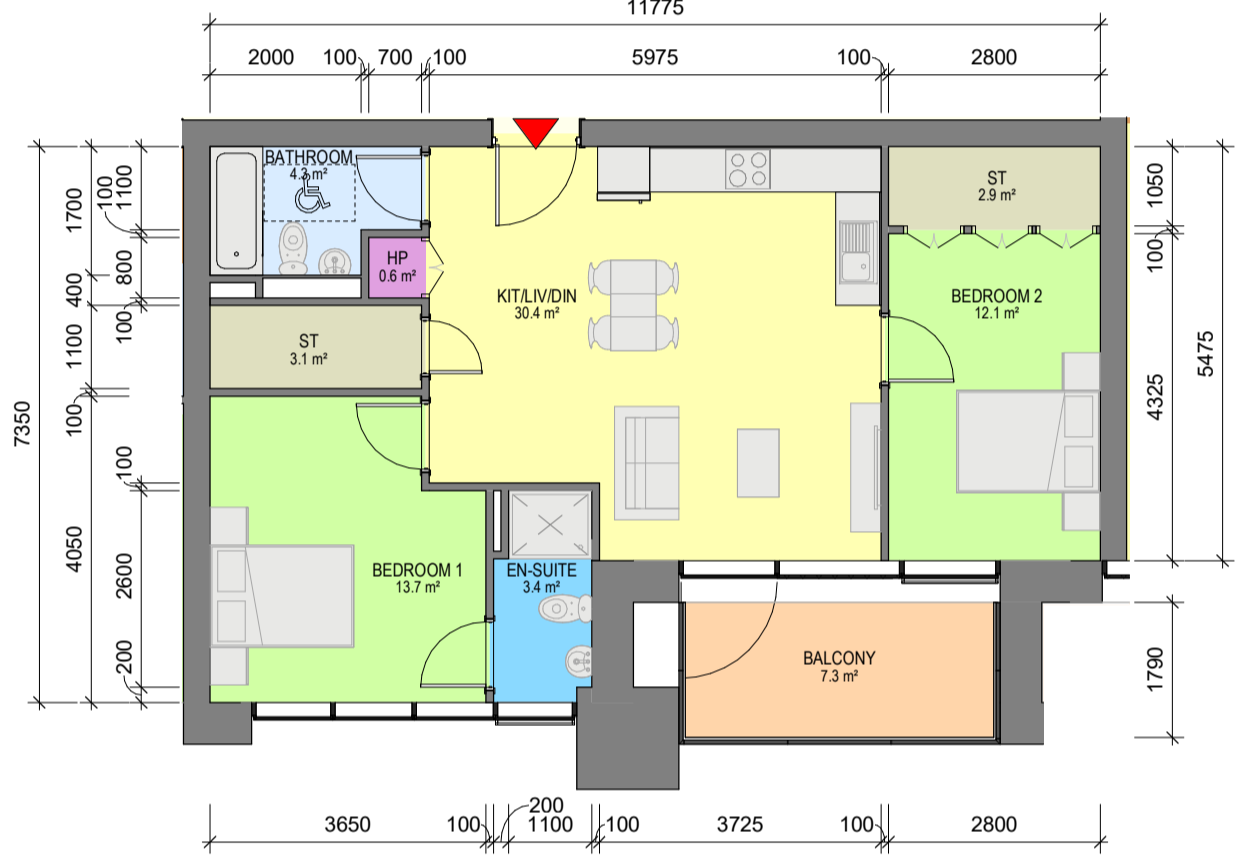
5 Apartment Type 2Q 1 : 100 - 2 BED, 4 PERSON APARTMENT - NET INTERNAL AREA (NIA) Areas shown in plan - GROSS INTERNAL AREA (GIA) : 73.90sqm
