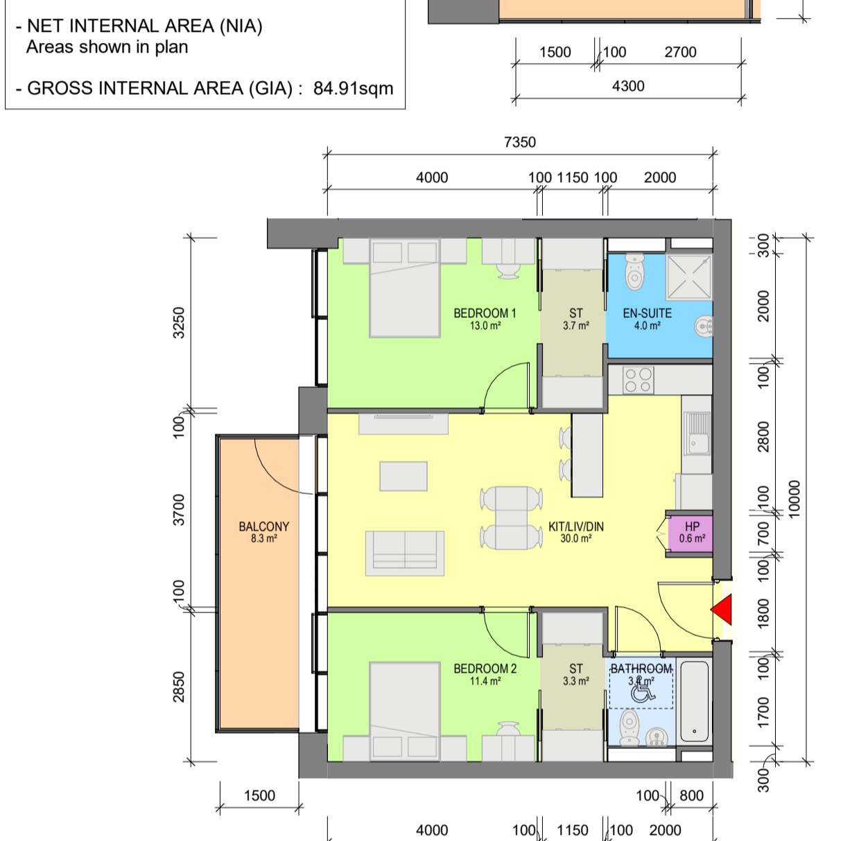
8 Apartment Type 2T 1 : 100 - 2 BED, 4 PERSON APARTMENT - NET INTERNAL AREA (NIA) Areas shown in plan - GROSS INTERNAL AREA (GIA) : 73.46sqm
