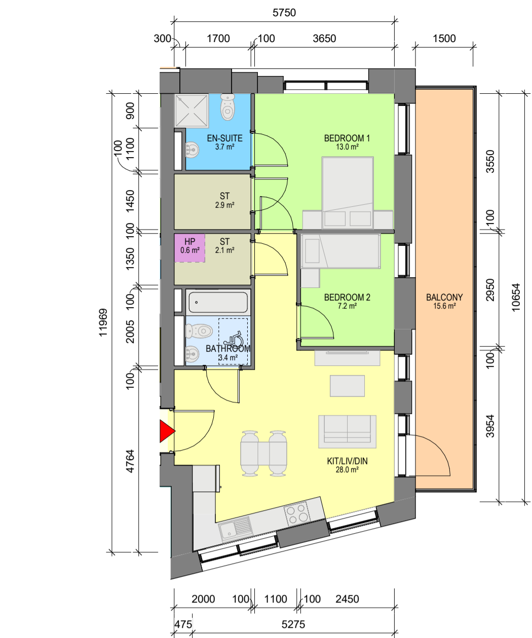
1 Apartment Type 2M 1 : 100 - 2 BED, 3 PERSON APARTMENT - NET INTERNAL AREA (NIA) Areas shown in plan - GROSS INTERNAL AREA (GIA) : 64.28sqm
