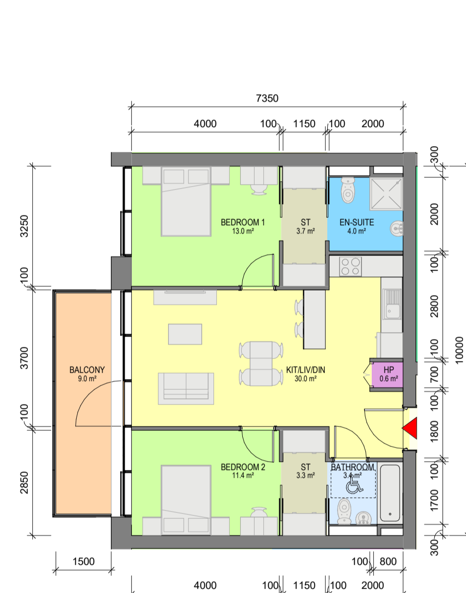
7 Apartment Type 2S 1 : 100 - 2 BED, 4 PERSON APARTMENT - NET INTERNAL AREA (NIA) Areas shown in plan - GROSS INTERNAL AREA (GIA) : 73.50sqm
